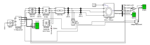
Fig.2 Simulation model of grid-excited induction generator
