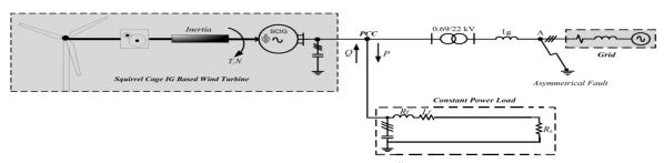
block diagram of GCIG with fault in grid side
